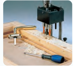
DRILLING JIG FOR CREMONE BOLTS Page 16.07
