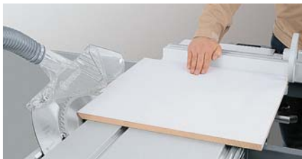
Tilt the saw blade to the desired angle, lay the workpiece against the crosscut fence.
