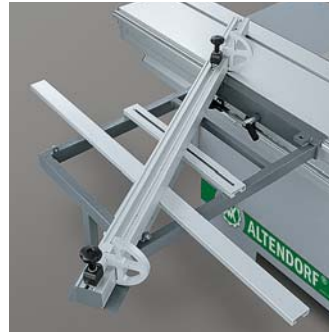
Crosscut-mitre fence: for accurate angle and mitre cutting in a single function. Cutting lengths: 105–2 600mm. Mitre angle infinitely adjustable by up to 49°.
