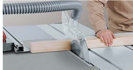
Position the rip fence in front of the saw blade, set to the required length and cut.
