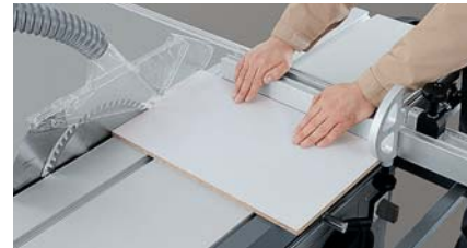
Cut the remaining piece to size on the crosscut fence.
