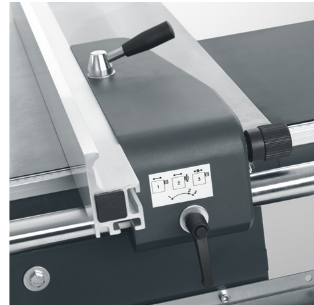
Rip fence with precise manual adjustment.
